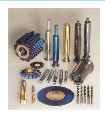
A Slovenian public research organization has developed several types of hard protective coatings to increase the lifetime of tools in machining. The benefit of deposited coatings is in their improved mechanical properties such as hardness, chemical inertness and adhesion. Partners that wish to prolong the lifetime of cutting and forming tolls are sought for commercial agreements with technical assistance.
